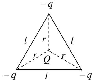
$$\text{据题意有 } 2F_2 \cos 30^\circ = F_1, \text{ 即 } 2 \times \frac{1}{4\pi\epsilon_0} \frac{q^2}{l^2} \cos 30^\circ = \frac{1}{4\pi\epsilon_0} \frac{qQ}{r^2}, \text{ 解得: } Q = \frac{\sqrt{3}}{3} q$$
